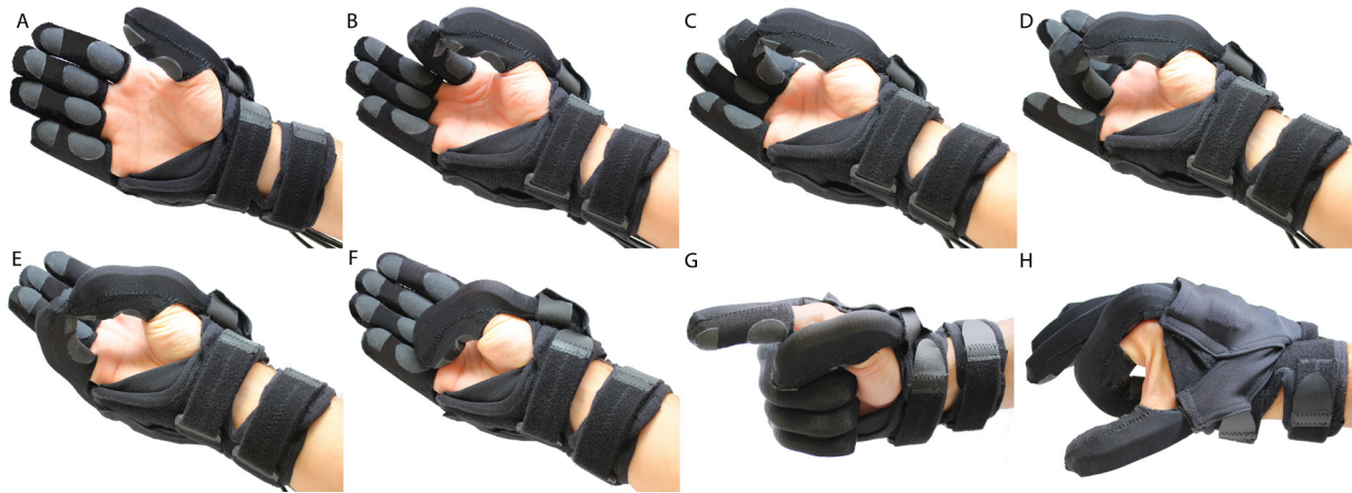
Figure 9. Range of motion of the soft robotic glove. A. Pretensioning of the fabric sleeves surrounding the fiber-reinforced actuators offers full hand extension. B-F. Executing the Kapandji test [21] with the soft robotic glove for thumb range of motion. G. Finger flexion with index finger straight. H. Index finger flexion.
