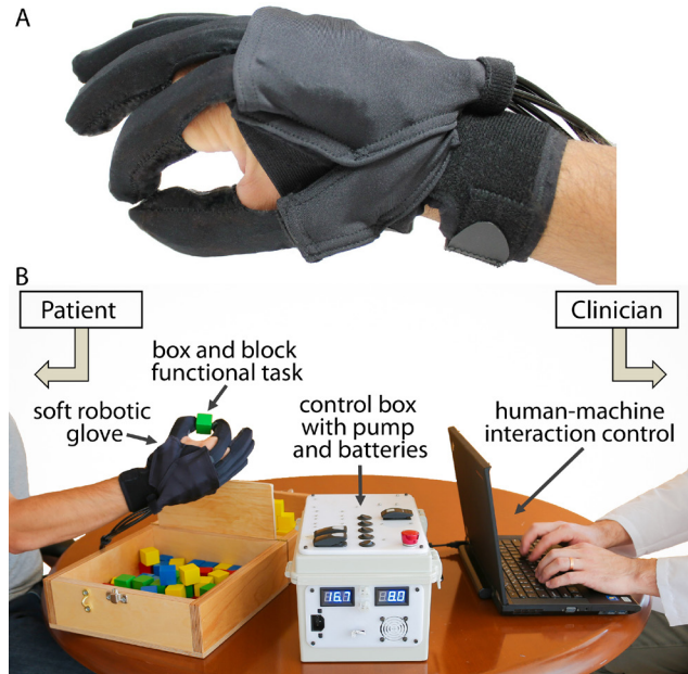
Figure 1. A. The prototyped hydraulically actuated soft robotic glove. B. Patient-clinician setup that utilizes the soft robotic glove to perform hand rehabilitation scenarios.
