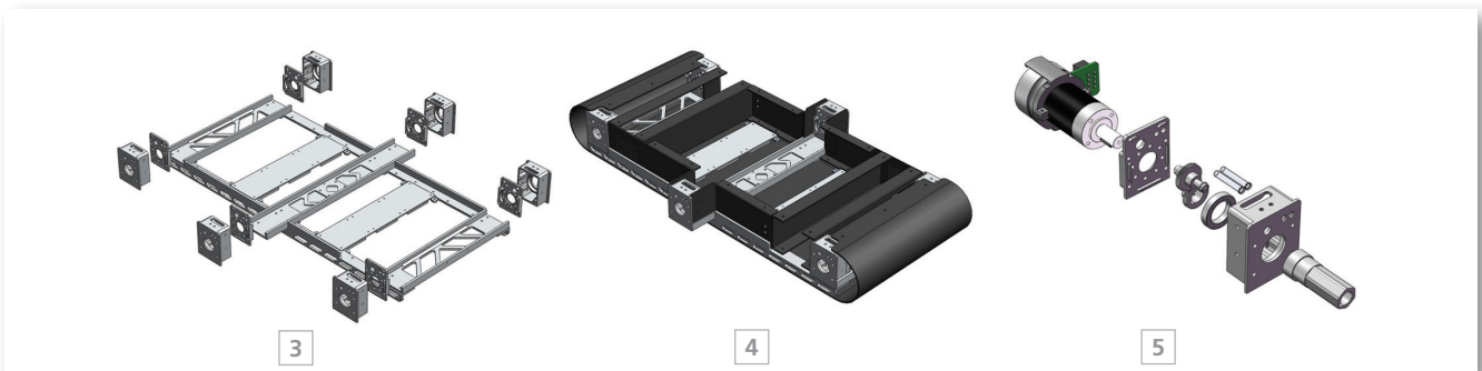
1 XRHex; 2 Side view of XRHex; 3 Model of aluminum frame; 4 Composite components added to aluminum frame; 5 Exploded view of motor mount assembly
